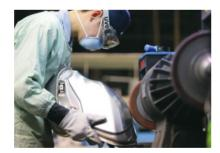
The fuel tank of the YZF-R1M flagship model is buffed to its final finish by a master craftsman
